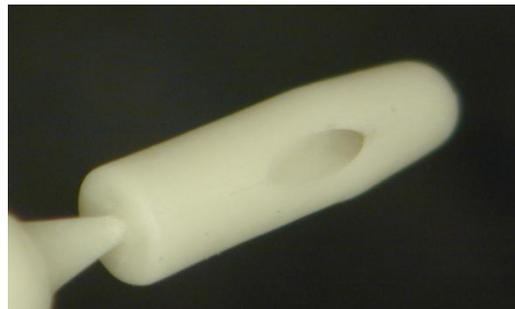
Figure 1.2 Vascular Closure Device with 50 µm (0.002") gate and 150 µm (0.006") suture orifice (photo courtesy of microPEP)
