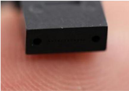
Figure 1.3: MES MT Ferrule Image on a Fingerprint. (Two 600 um holes and twelve 125 um holes shown on face)
