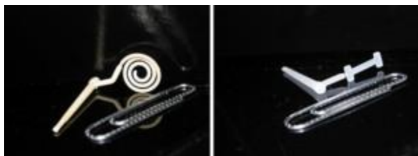
Figure 1.4 Spiral Flow Test and Micro Tensile Test Bars
