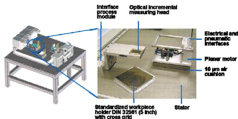
Figure 1.6 The Mini-Pod System, photo and concept courtesy of the Fraunhofer Institute, Stuttgart, Germany.
