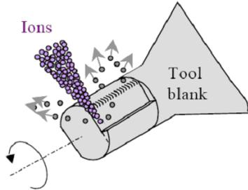
Figure 1.4-Schematic of ion beam sputtering technique-Photo courtesy of Sandia National Laboratories, Livermore, CA
