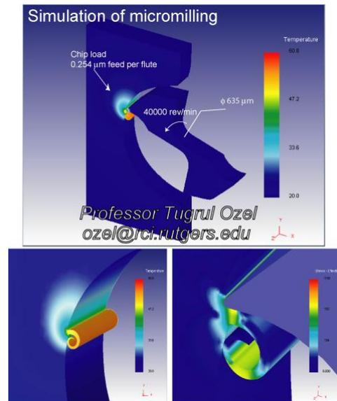
Figure 1.2 Simulation of End Mill Temperature Gradient, photo provided by Rutgers Engineering
