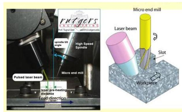
Figure 1.3 Photo and close-up depiction of Laser-Assisted Micro Milling, photo provided by Rutgers Engineering
